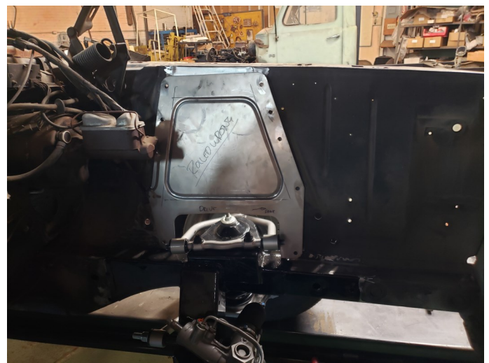
New inner fender filler panel. Rolled center for extra support
