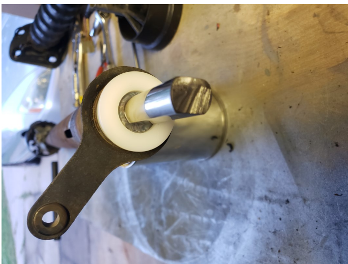
Had to make a steering column bushing to center steering column shaft.
