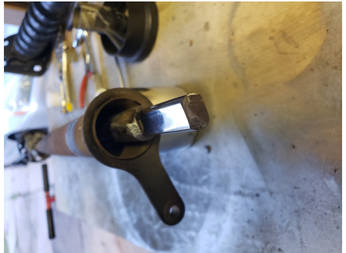
Steering column had to be removed and disassembled for new double D shaft to be welded for new steering column u joints
